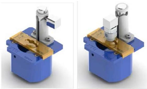
Place the "Holder XTU Insert microTUBE 15 μL" (PN 500420) in the Holder XTU, you should feel the magnets contact
